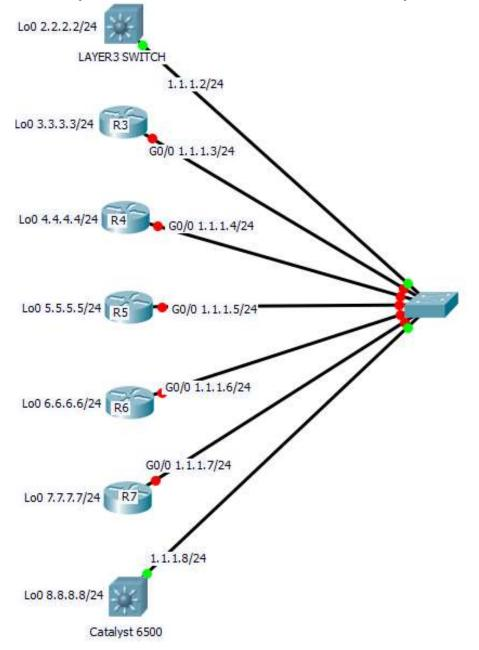
Topology for the first step of the lab which is to establish end-to-end connectivity via full mesh:
